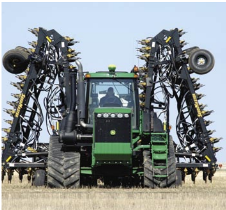
The 80-foot unit folds into the same width as other Seed Masters for transport.
