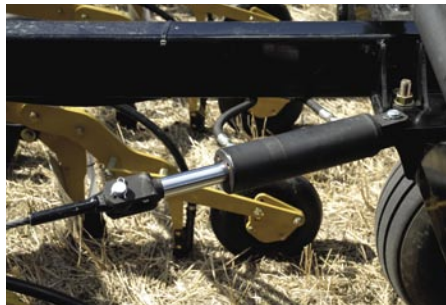
The active wing brace bolsters the frame strength on the 80-foot Seed Master.
