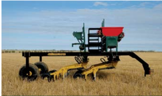
Seed Master's New Plot Seeder - Eight openers slide on a track and are pinned into position, for quick and easy row spacing changes.
