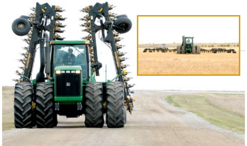
Narrow Folding Air Drill - Seed Master's new Compact-In-Transport line offers drills up to 70-foot wide (shown here) that fold to 18 feet for transport.
