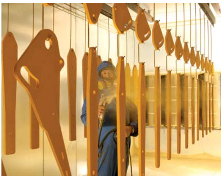
Lean Manufacturing means all components for one Seed Master advance through the manufacturing process together. Here, powder coat paint is applied. The next step is a large oven where the paint is baked on for a superior finish.
