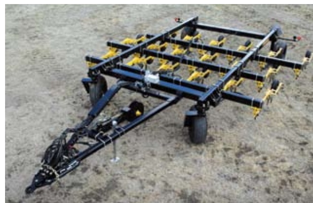
AAFC's new SeedMaster plot seeder (shown here before the tanks and Individual Row Metering were installed) will be used to advance tall stubble research.
