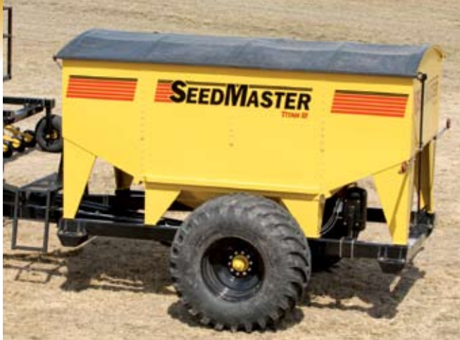
The new Titan III fertilizer tank offers a 600-bu capacity (top) and easily converts to a grain cart at harvest (bottom).
