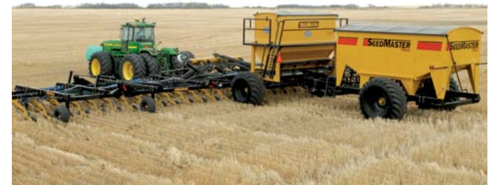
The new Titan III fertilizer tank combines with SeedMaster's on-board seed tank to provide a 920-bu carrying capacity - the largest in North America.
