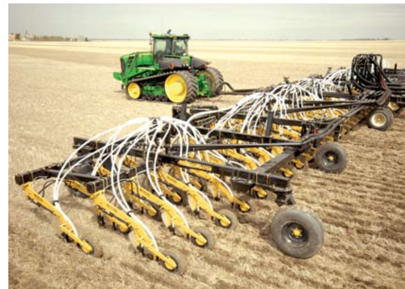
SeedMaster's New FLIP System takes a new and simple approach to implement overlap - almost completely eliminating costly overlaps - without lifting openers from the ground.
